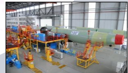
Stations 42 / 41 Preparation / fuselage join-up
